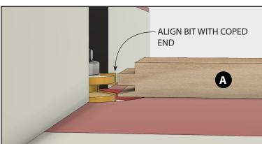
Remove the coping bit and replace it with the profile cutter. Place one of the coped rails face down on the table and adjust the bit's height so that the cutter aligns with the cope in the end of the rail.
