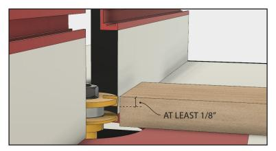
When using any rail-and-stile router bit set, it's always a good idea to make the cope cuts first. Insert the coping bit in your router and set the height so that the slot cutter makes at least a 1/8" deep cut into the stock.
